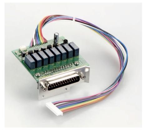
Relay output to connect relays, signal lamps, valves etc., 5 outputs for weighing in 3 tolerance ranges, must be ordered at purchase
