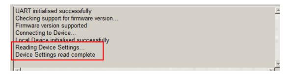
In case of errors, make sure that the DCE-DTE switch is set to DCE and the communication parameters match with the actual adapter settings. If no connection can be established, please reset the adapter to the factory settings (see above).
